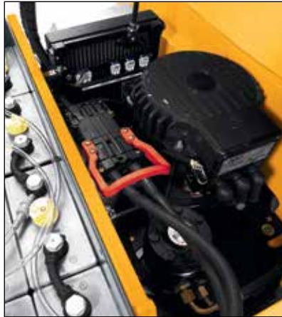
Drive and lift motor with AC technology
